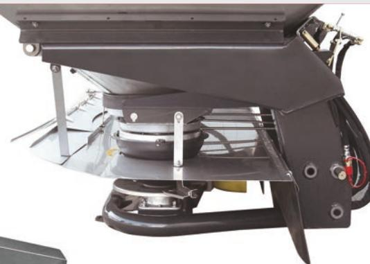
**Frame:** structural strength with useful loads up to 3600 kg. I and II category hook and versatility hooking in three different positions; normal, 100 mm moved; or 150 raised for late injections.
