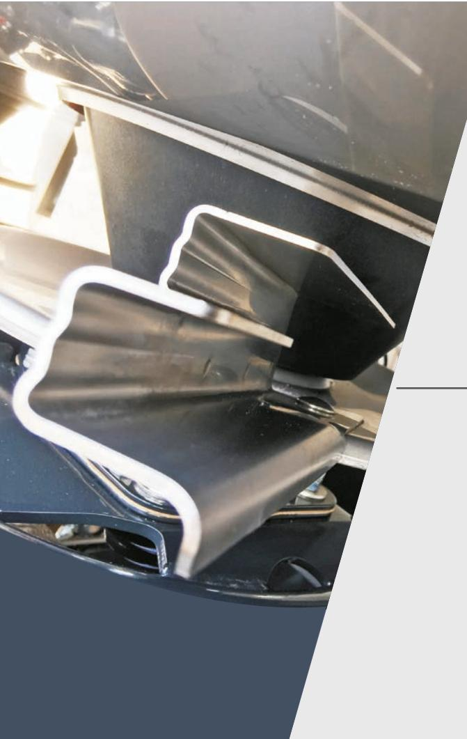
Feed the fertilizer laterally to the vane, **means elimination of the granule brake and powdering** during distribution.
