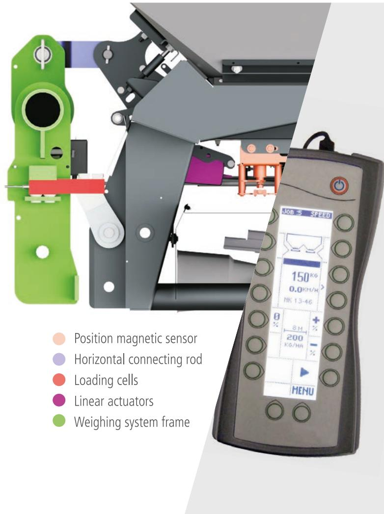
The required dosage **is automatically adjusted according to the forward speed** (Forward Speed Calibration) by means of two linear actuators. The system enables the instantaneous **variation** of the applied dosage, the **interruption of spreading on one side**, the **verification of the quantity and worked hectares** directly and comfortably from the tractor's seat.
