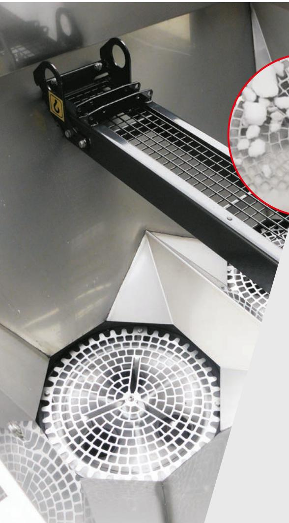
The system with vibrating hopper bottom that feeds continuously the distribution system. The non-use of agitators avoids the products crushing, assuring a **uniform dosage of the chosen quantities**, of granular, powdered and pelleted fertilizers and seeds.
