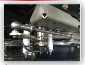
Two magnetic sensors detect the exact opening of each shutter and control directly the linear actuators avoiding any possible error of position.
