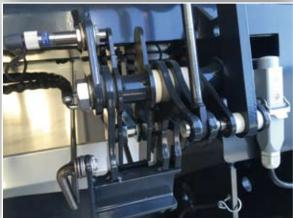
Two position sensors detect the ON/OFF status of the hydraulic system and therefore the distribution. In order to avoid spreading beyond a field limit, the GPS transmits the signal of distribution start after the tractor has run a distance from the beginning of the field equal to the spreading width of the fertilizer spreader.
