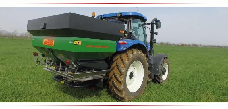
The "W" versions of the CRONO and ELETTRA fertilizer spreaders with electronics for the forward speed calibration integrate a weighing system that enables to check the exact delivered quantity per hectare.
